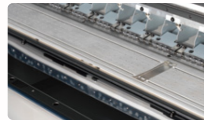
Platen with Adsorption Function (for transfer paper)
