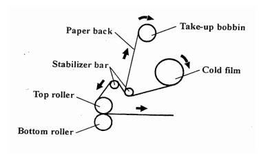
• Slide the cold film onto the roll shaft. Hold the cold film on the core adaptor to prevent it rotating. Screw the bolt on the core adaptor, put the roll on the brackets. Make sure both ends are fitted securely.
